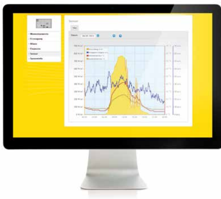
Daily overview with wind sensor (blue), module temperature (red), ambient temperature (green) and yield curve (yellow).
