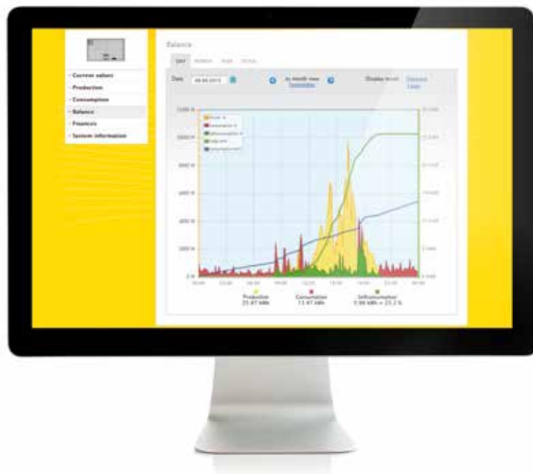
The generated output and the power consumption of the PV plant are displayed in the “Balance” section.
